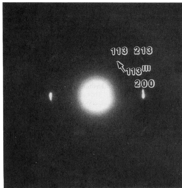
Figure 3. Tilted ED pattern along the [031] zone for PEKK(T/I) crystallized at 260 °C for 60 min from the melt.
